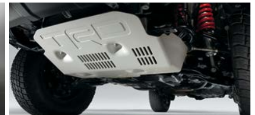
TRD-stamped aluminum front skid plate
